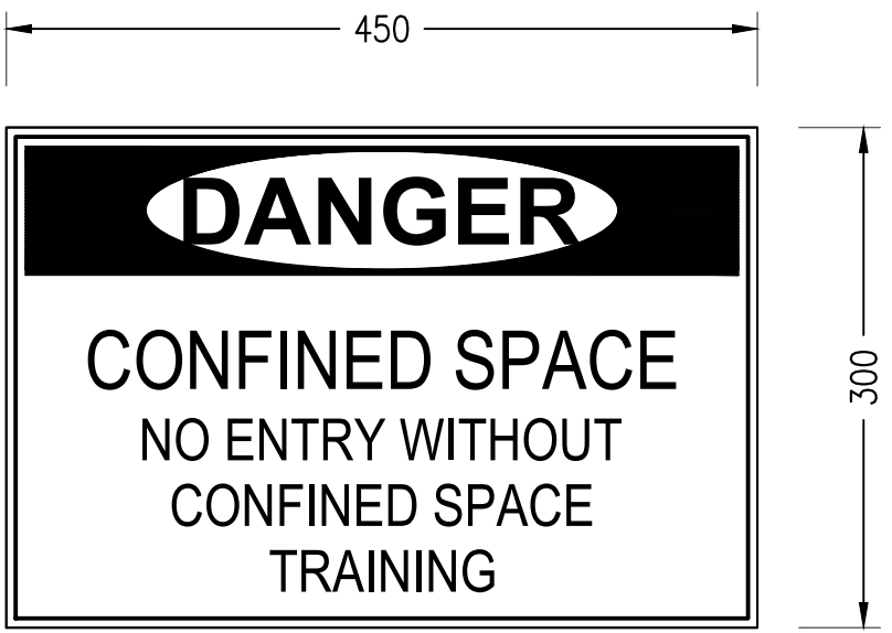
CONFINED SPACE SIGN DETAIL SCALE 1:20
